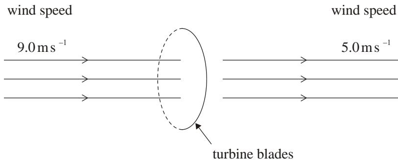
The density of air immediately after passing through the blades is  $2.2 \text{ kg m}^{-3}$ . The turbine and generator have an overall efficiency of 72%.
